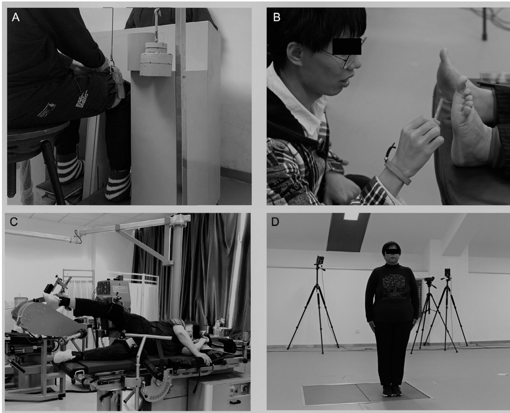
Fig. 2. Test illustrations: (A) the proprioception test using a proprioception test device, (B) the cutaneous sensitivity test with a set of Semmes–Weinstein monofilaments, (C) the muscle strength test using the IsoMed 2000 muscle strength testing system, and (D) the center of pressure test on a KISTLER force plate.
