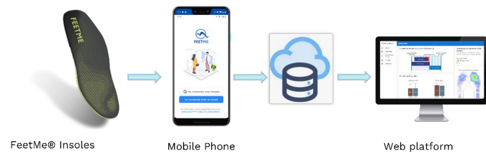
Figure A1. FeetMe® Monitor solution includes the insoles, and the mobile application to collect data and to transfer to the web platform. The web platform shows the gait parameters and the pressure measurements.
