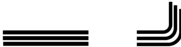
Figure 3. Interlaminar sliding caused by laminate folding.
