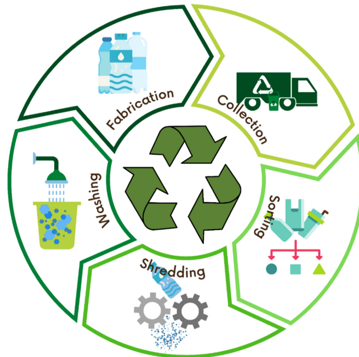
Figure 2. Overall mechanical recycling process of waste plastics.
