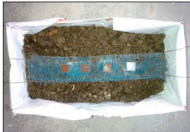
Figure 5. Compost box with samples placed inside.
