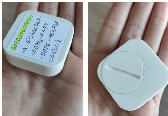
Figure 4. iB004N beacons used for beacon-based localization.
