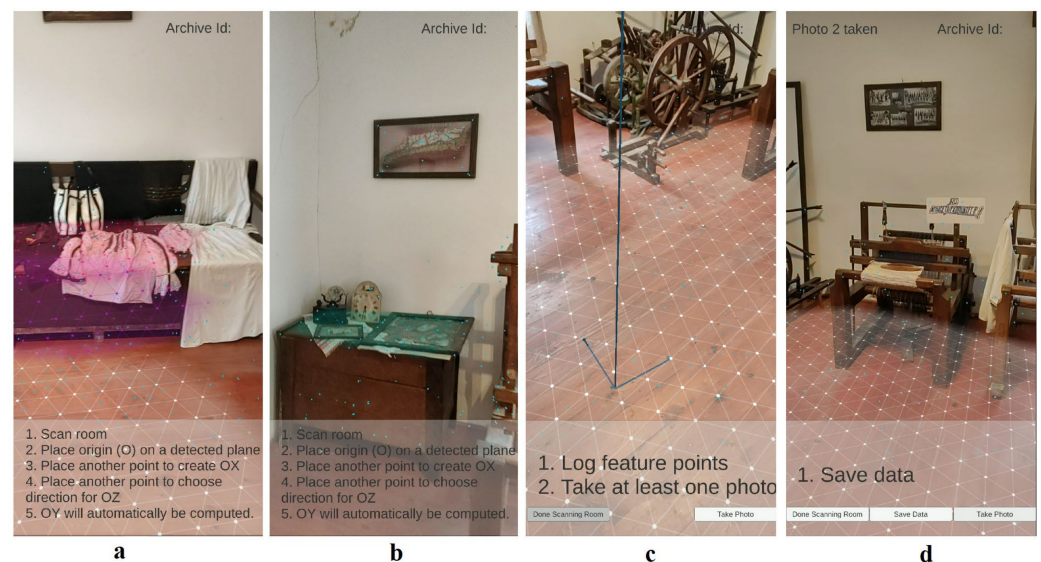
Figure 3. Workflow of the location manager application displaying the guidelines and several prominent planes: the floor and several planar surfaces of a bed (a), displaying detected feature points (b), displaying the user-defined coordinate system (c), and displaying a message that a photo has been taken (d).
