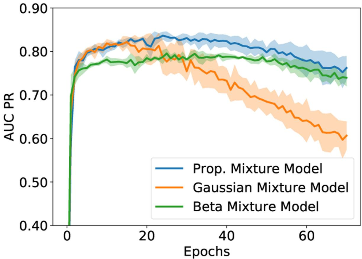
**Fig. 6:** AUC PR obtained with alternative mixture models for modeling the loss distribution as a function of training epochs. The curves show the average AUC PR values over 5-fold cross-validation, and the shaded region represents the one standard deviation from the mean AUC PR values.
