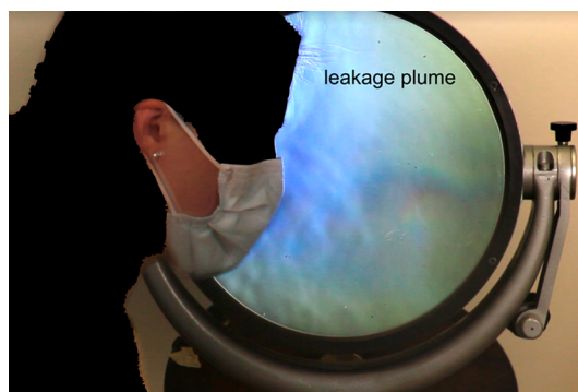
Figure 7. Observed leakage plume.
