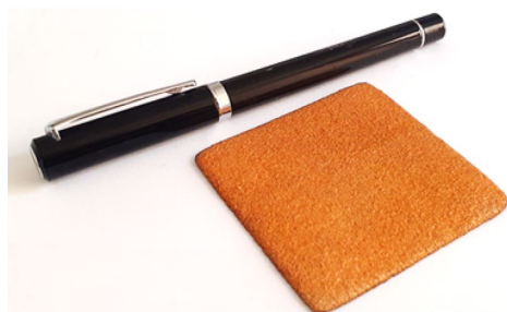
Figure 8. Fabricated three-layer radiation shield sample.
