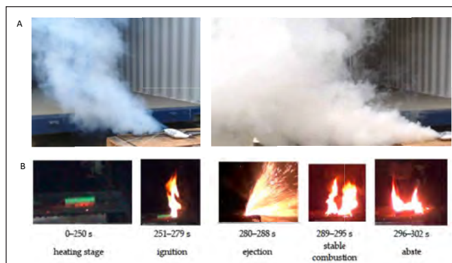
Fig. 7 - Thermal Runaway and Gas Release. A) Illustrates the ejection phase of thermal runaway where high pressure gases including hydrogen fluoride gases are vented; B) Time rendered photo-capture of the thermal runaway process. Notice that combustion may or may not occur during the ejection phase as compared to A. Image reproduced with permission from Wang et al. 20
