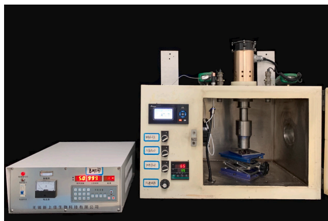
Fig. 1. Air dryer coupled with ultrasound device used for blackberry drying.
