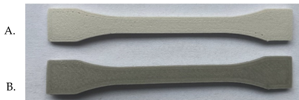
Figure 15. Samples for strength tests: (A). PA12- \text{ZrO}_2 , (B). PA12- \text{Al}_2\text{O}_3 .
