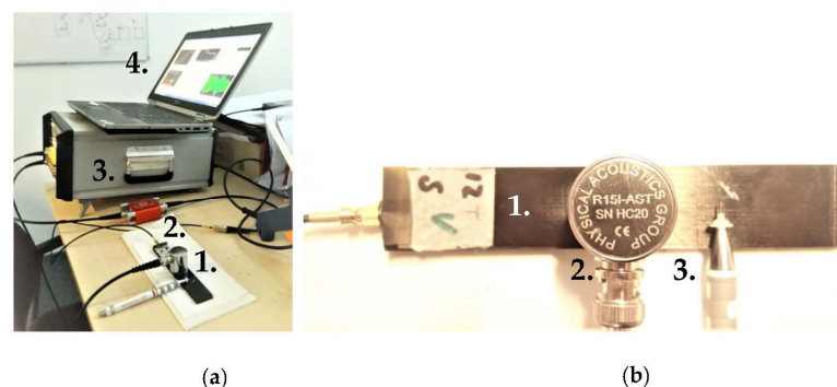
Figure 2. Set-up for exciting and measuring a Hsu-Nielsen source [36]: (a) Overview of the set-up, with the numbers 1 to 4 corresponding to the specimen, AEP-5H preamplifier, AMSY6 data acquisition system and a measurement computer. (b) Close-up showing the specimen (1.), AE sensor R15I-AST (2.) and a mechanical pencil with Nielsen shoe (3.). Note that in the final assessment a pencil with 0.5 mm diameter lead was used at a distance of 60 mm from the centre of the sensors.
