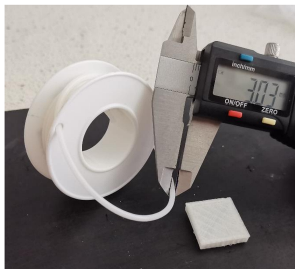
Figure 11. Photography of the produced COMP-7,5PLA filament and printed cube.
