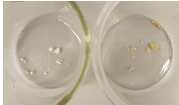
Figure 12. Photo of amikacin samples after heat treatment, after 10 min (left) and 30 min (right) at 195\text{ }^{\circ}\text{C} .
