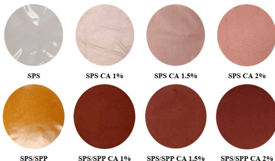
Figure 4. Visual appearance of SPS and SPS/SPP films at CA of 0, 1, 1.5, and 2%. Reproduced with permission from Ref. [52]. Copyright 2021 Taylor & Francis.
