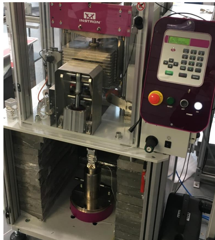
Figure 8. General view of dynamic testing machine Instron Ceast 9450 HES.
