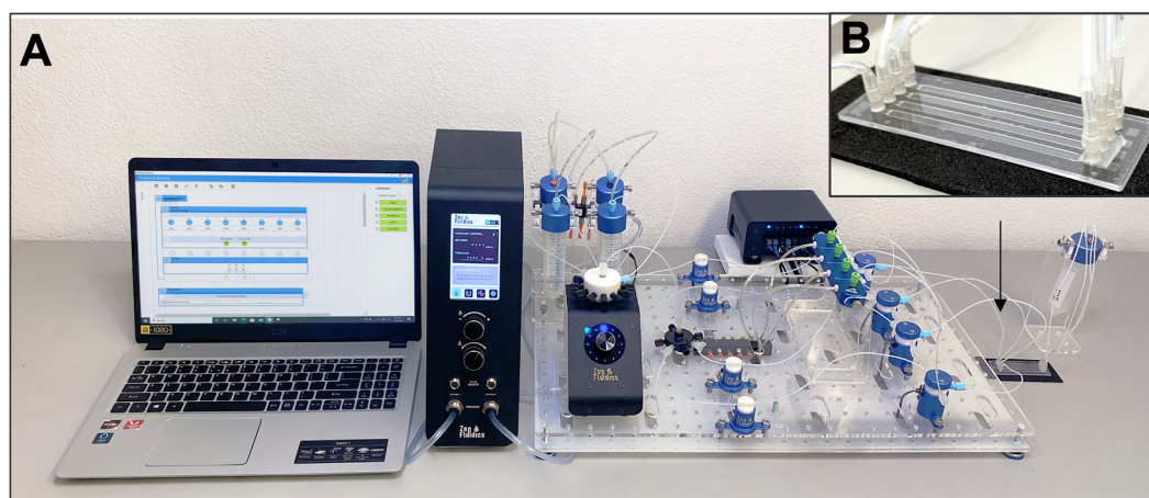
Figure 2. (A) Photograph of the experimental setup of our automated ELISA on-chip. (B) Picture of the microfluidic device used in our setup.
