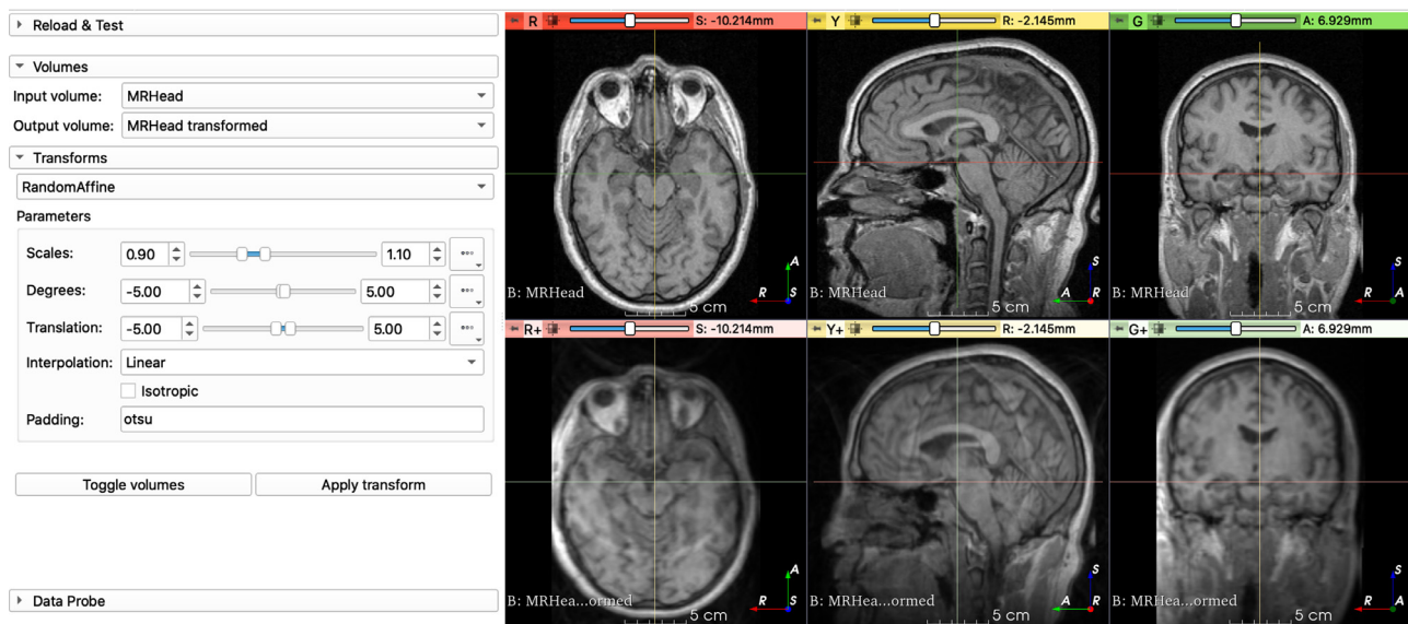
Fig. 7. GUI for TorchIO, implemented as a 3D Slicer extension. In this example, the applied transforms are RandomBiasField, RandomGhosting, RandomMotion, RandomAffine and RandomElasticDeformation.
