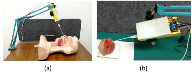
Fig. 9. Experimental setups for (a) the phantom and (b) the pig nose tests.
