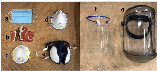
FIGURE 16. Different face covers tested: (a) surgical mask; (b) handmade mask; (c) FFP1; (d) FFP2; (e) respirator; (f) university-made lightweight face shield; (g) commercially heavy-duty face shield.
