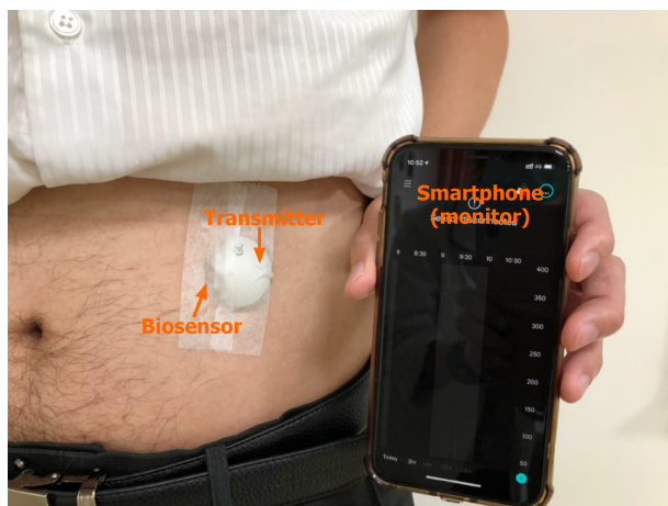
Figure 1 Three major components of the real-time continuous glucose monitor.
