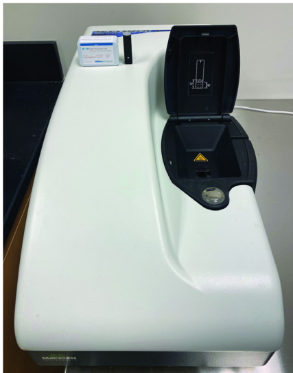
Figure 2. Zetasizer Nano S particle size analyzer. The ZEN2112 cuvette is shown next to the open sample compartment.
