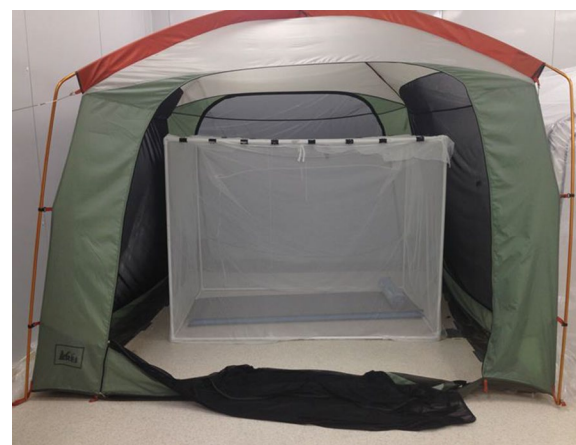
Fig. 1 REI® tent with untreated bed net fastened to a PVC frame with paper clamps. Cameras and CPU fan not present
