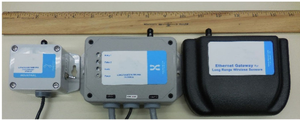
Fig. 2. IoT system sensor, control node, and gateway (left to right)
