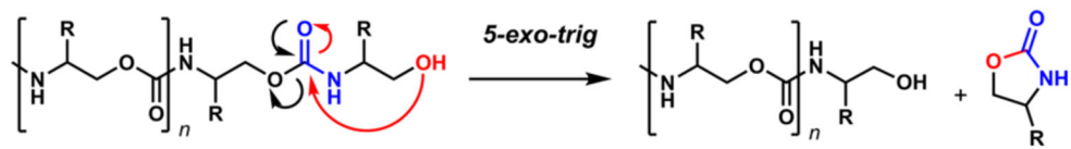
Scheme 1. Self-Immolative Mechanism of Urethanes
