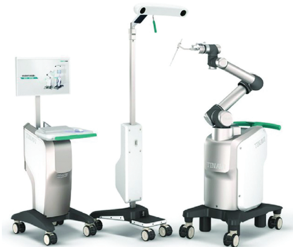
Figure 2. The TiRobot. The TiRobot consists of a planning station, optical tracker, and a robotic arm to assist with surgical guidance. Figure previously published under a creative commons licence. [34]
