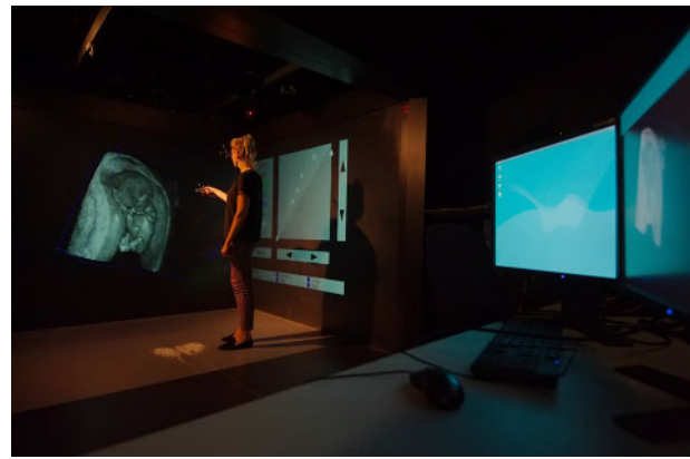
Figure 3 I-Space virtual reality system. A fetus of 12 weeks' gestational age is displayed on the front wall. The researcher is wearing 3D glasses to observe real depth perception and interact with the dataset by using a joystick. Be aware that real depth perception cannot be shown on paper
