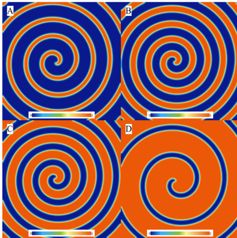
Figure 11: Spiral wave in the Barkley model initiated when the parameters of the Eq. (9) were set to a = 0.5 , b = 0.04 , and \epsilon = 0.02 (panel A ). Then, parameter a of the model was slowly and interactively changed to 0.8, 1.0, and 1.2 from B to D . Note how the wavelength increases as a is increased.
