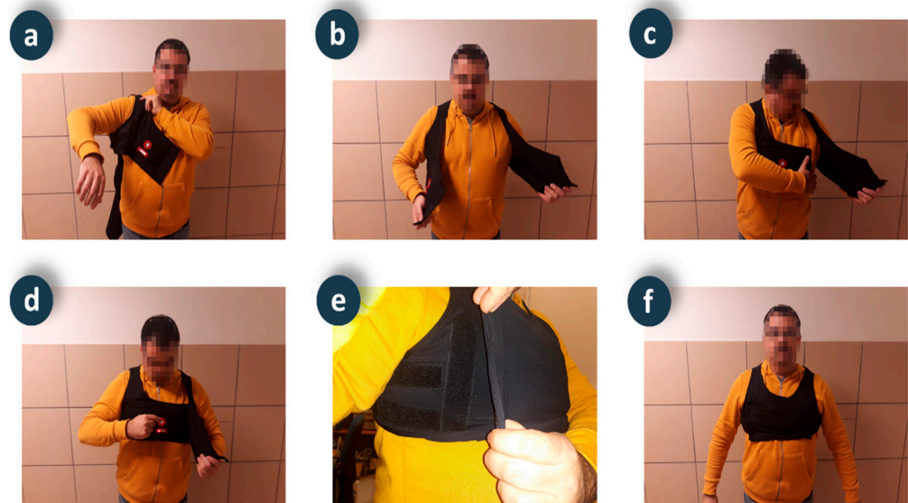
Figure 6. Sequence of the smart vest placement and activation process.
