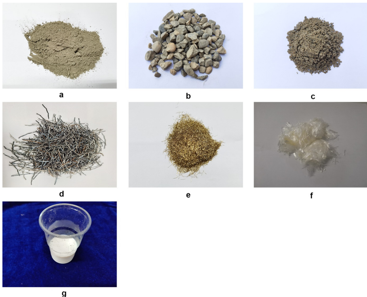
Figure 1. Raw materials: (a), ordinary 42.5 silicate type Huaxin Cement; (b), cobblestones with a maximum nominal grain size of 10 mm and a grading of 5–10 mm; (c), fly ash; (d), ordinary steel fiber; (e), ultrashort ultrafine steel fiber; (f), polypropylene flexible fiber; (g), polymer emulsion.
