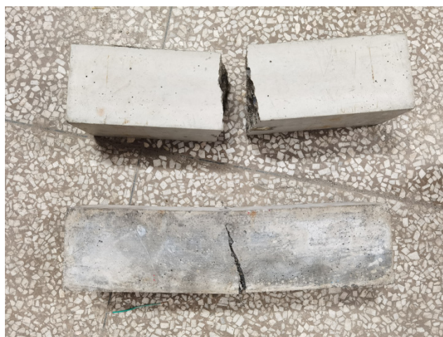
Figure 6. Failure modes of the plain concrete and hybrid fiber–polymer concrete.
