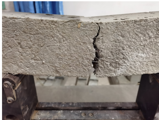
Figure 7. Details of crack resistance by the hybrid fiber–polymer concrete.
