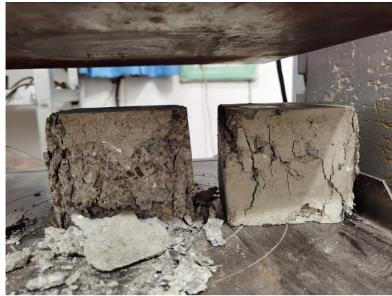
Figure 5. Comparison of compression failures in the plain concrete (left) and hybrid fiber–polymer concrete (right).
