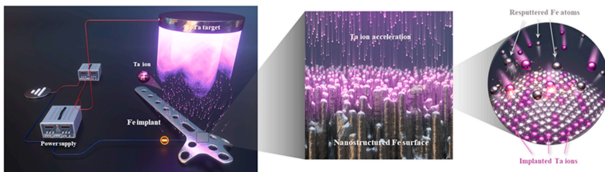
Fig. 8. Schematic diagram of the TIPS process for Fe implants with Ta sputter target and negative substrate bias voltage of 1000 V.
