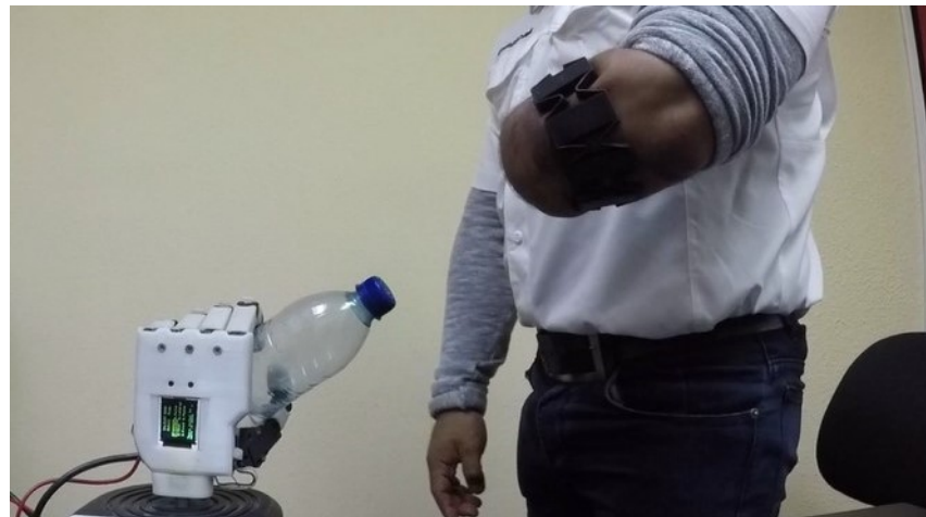
Figure 10. A limb-impaired volunteer testing the UPI with the reduced contraction set of muscles.
