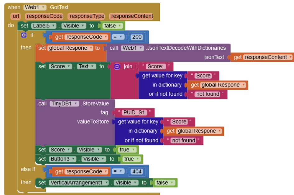
Figure 5. In this block, the application reads the web response and stores it in the phone's memory, where it can be uploaded later. The simplicity of block-based coding makes it available for use and editing without the need for a skilled technician.
