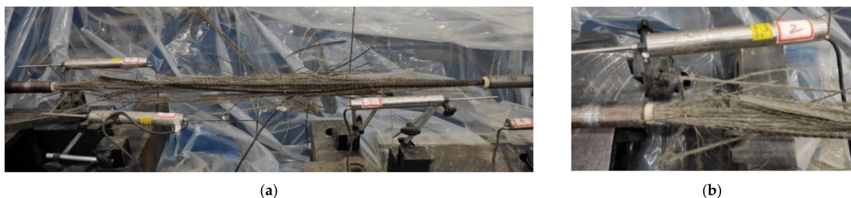
Figure 4. Fracture of the BFRP tendon: (a) failure mode; (b) anchor without obvious slip.
