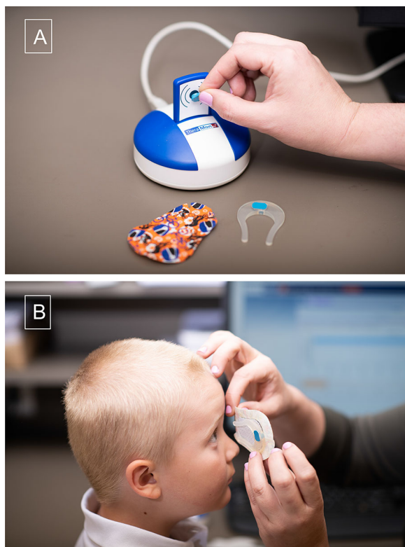
Fig. 6 The temperature-sensitive Theramon ® sensor is fit into a horseshoe shaped silicone Eye Patch Assistant (EPA) [47], which can then be placed on an adhesive eye patch, shown next to sensor reading device (a). Also shown is the EPA with a microsensor in place on the eyepatch, ready to place over the child's eye (b)
