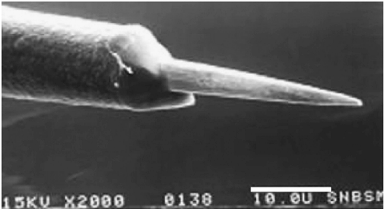
Figure 6. SEM image of a microwire probe tip. A 70%/30% platinum/iridium wire is electrochemically sharpened (producing the pointed tip), then coated with parylene C. After coating, the electrode tip is exposed using laser etching. Reprinted from [8], Copyright (2007), with permission from Elsevier.
