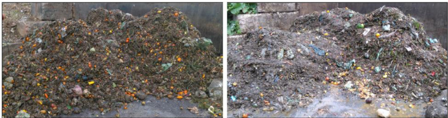
Fig. 7. Rural organic fraction of municipal solid waste (OFMSW) in January (left) and in June (right) as an example for the organoleptic examination as described in Fig. 6.
