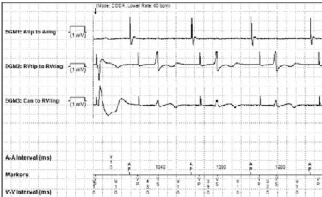
Figure 2 Device interrogation obtained while in emergency department showing atrial capture with prolonged AV conduction delay resulting in first-degree AV block with intermittent ventricular noncapture.
