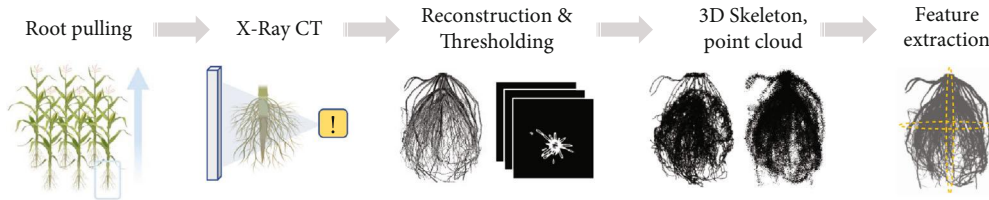
FIGURE 1: Pipeline for 3D root imaging using X-ray computed tomography. Samples are excised from the soil in the field using the root pulling force method, and the measurement is recorded. The root crown is washed, dried, and then imaged using the NorthStar Imaging X5000 (see Methods) to generate radiographs as the sample is rotated 360° across the vertical axis. From the radiographs, a 3D reconstruction is generated using the FDK algorithm. Slices along the vertical axis are exported for automated thresholding, from which a skeleton and point cloud model of the root crown are generated. 3D root traits are then measured from the skeleton and point cloud and analyzed.
