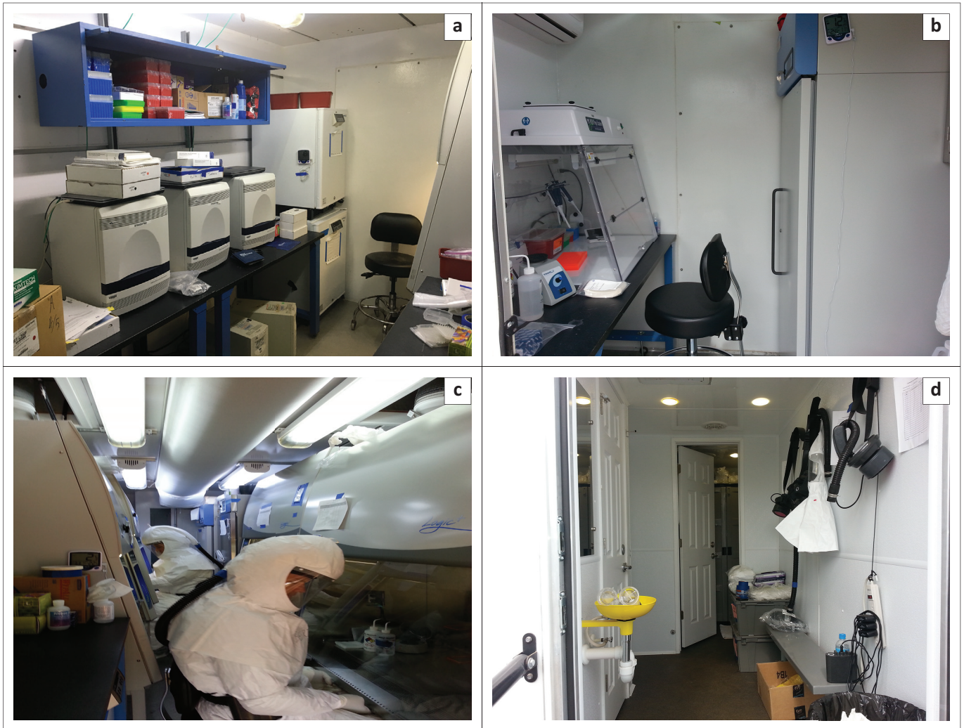
FIGURE 1: MRI Global mobile diagnostic laboratory that was deployed in response to the West Africa Ebola virus outbreak. (a) Interior of polymerase chain reaction laboratory unit. (b) Interior of master mix laboratory. (c) Interior of inactivation and extraction laboratory unit. (d) Interior of locker room.
