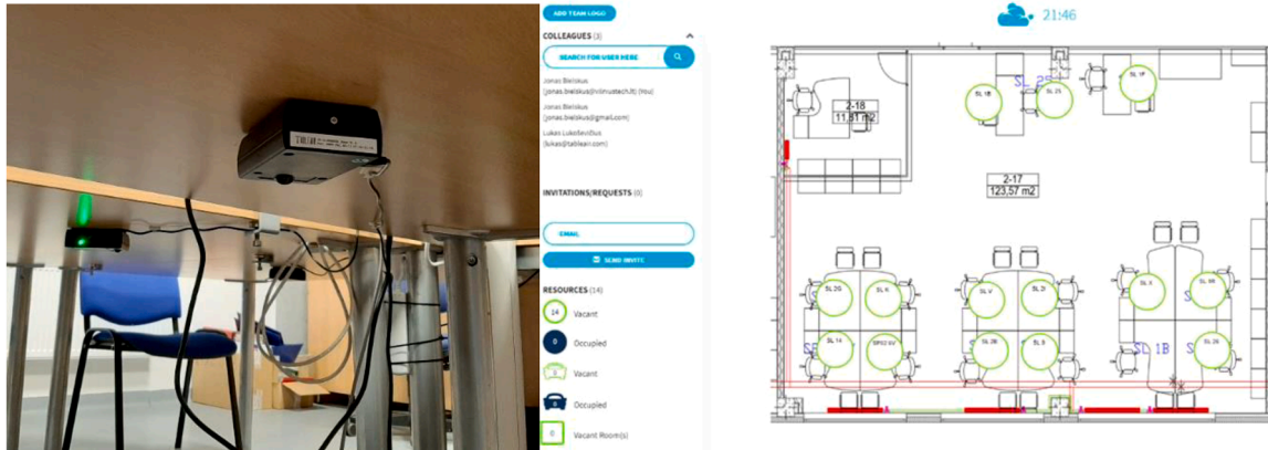
Fig. 4. Measurement of desks occupancy with PIR + temperature sensors.
