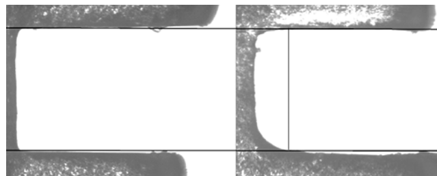
Figure 6. A right and left central incisor bracket from the same series. Not only would the same full-size wire not fit into the slot, a first-order discrepancy would also be introduced, due to a rounded lower corner on the right bracket.
