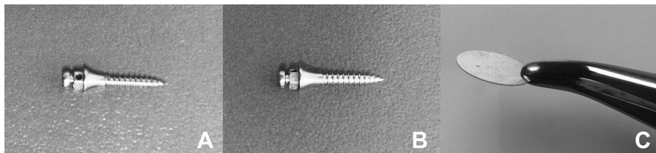
Figure 1. Materials investigated. (A) Morelli mini-implant. (B) Neodent mini-implant. (C) Polystyrene, used as control.
