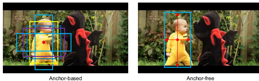
Figure 1. The left side is the anchor-based method which uses the fixed different ratio aspects anchors to locate the location of an object, and the right side is the anchor-free method that directly estimate the bounding box.
