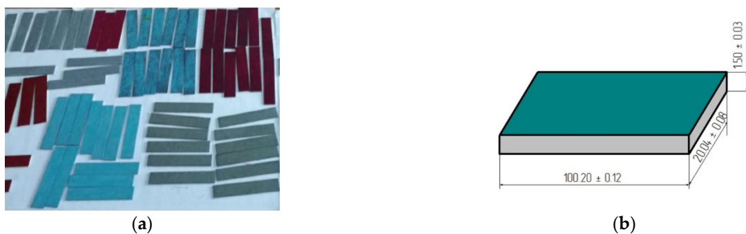
Figure 1. Sample of steel sheets with varnish coats: (a) view of samples of steel sheets with coatings; (b) scheme and dimensions of a steel sheet sample in mm.
