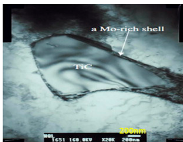
Figure 7. TEM bright field image showing a Mo-rich shell around TiC in Al-alloy (Al–0.6Cu–0.6Mg–1.2Si–0.25Mn–10TiC–1Mo). Reprinted from Ref. [92] with permission from Chem. Eng. J.
