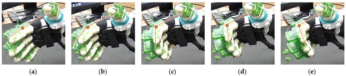
Figure 18. Fingers' PIP flexion: (a) index, middle, ring, and small finger PIP joints are extended, PIP joint angle: 0^\circ ; (b–d) intermediate PIP joint positions; and (e) PIP joints are flexed, PIP joint angles: 80\text{--}82^\circ .
