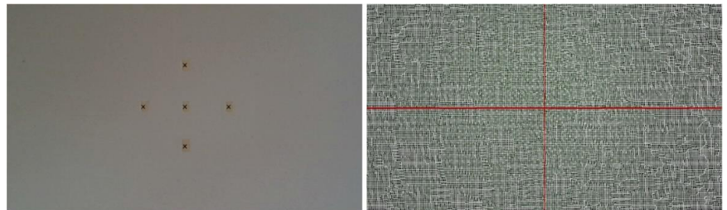
Figure 10. Acquisition setup to ensure camera-plane perpendicularity during the systematic depth error evaluation test.
