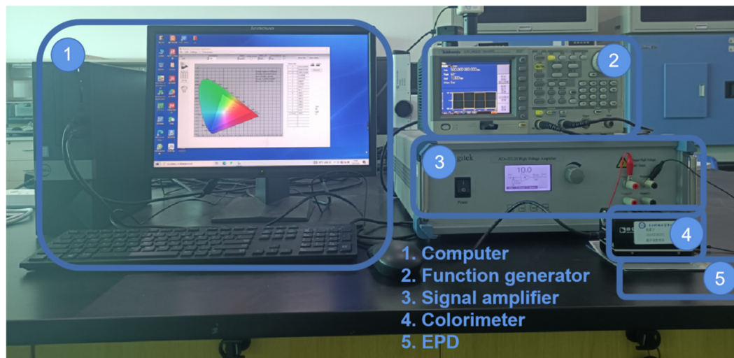
Figure 2. Experimental platform for the testing of EPD color gamut, luminance and response time. It was composed of a driving system and a testing system. (1) computer. (2) function generator. (3) signal amplifier. (4) colorimeter. (5) EPD.
