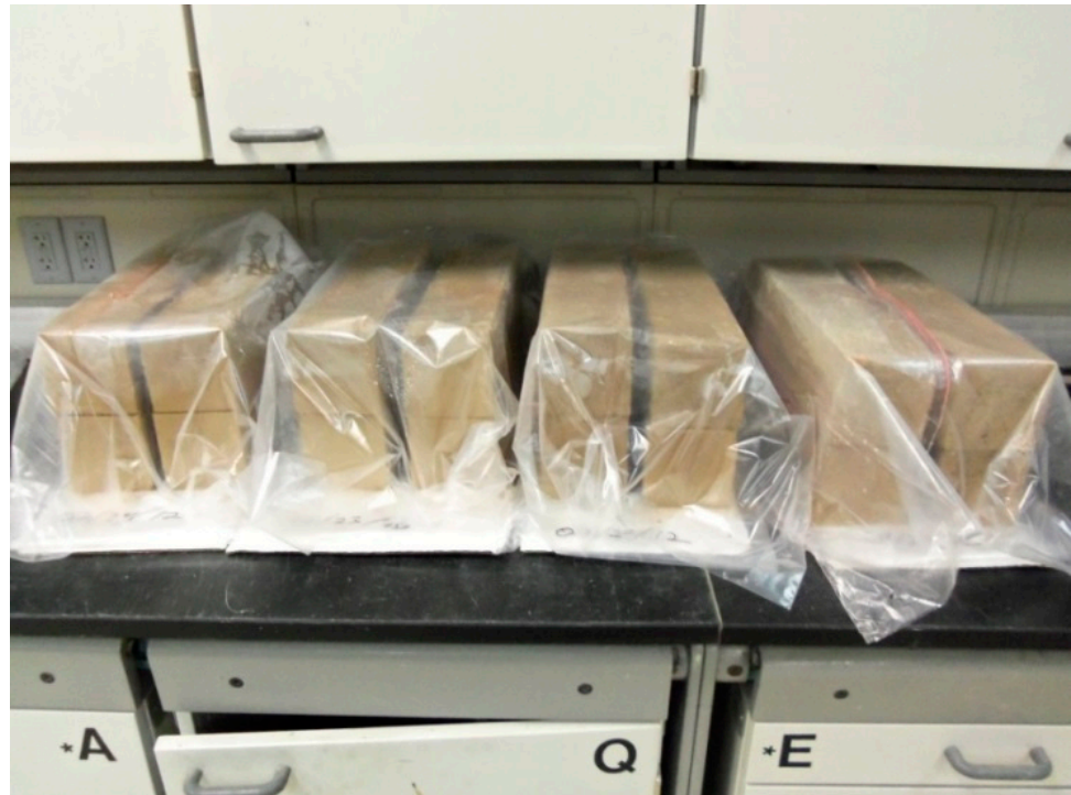
Figure 2. Initial cure of CEBs under plastic sheets.
